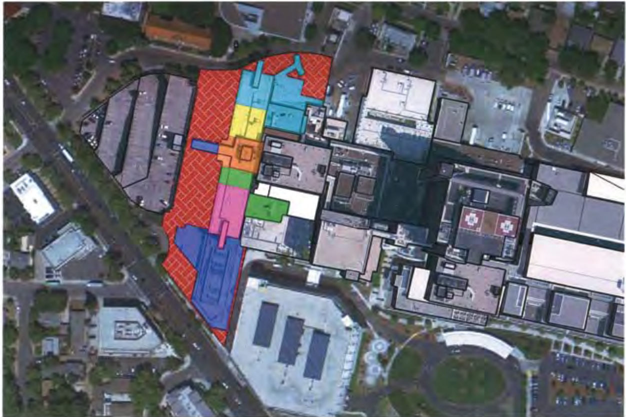
Phase-5 North-South Tower Abatement and Demolition Sequence Plan
